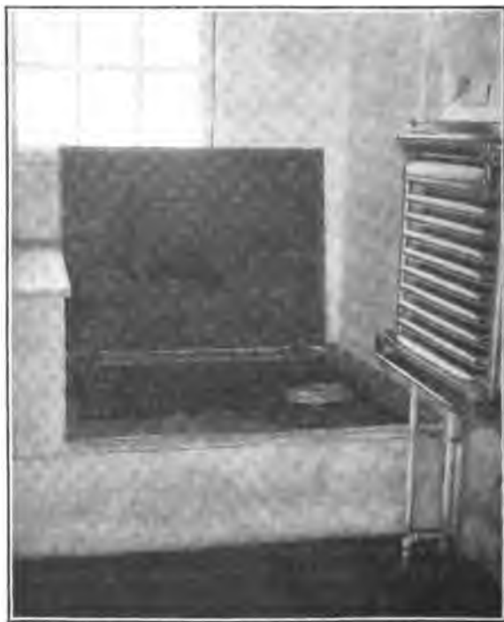
FIGURE 6.—Milk cooler and concrete tank for cooling and storing milk and cream
